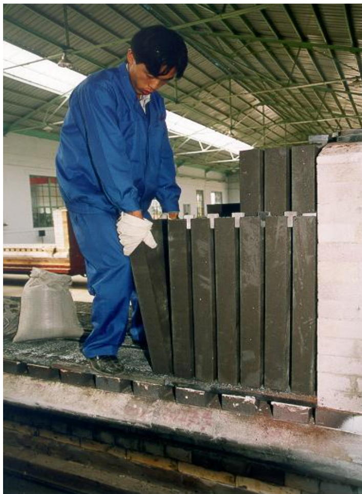
Blocks being placed in the kiln cars before going into the nitride furnaces.
