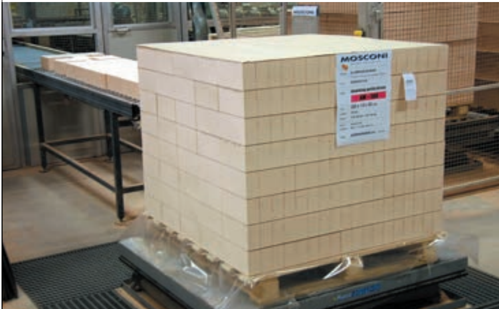
A pallet with Mosconi's newly developed msb AW-500 insulating brick. A brick developed especially for pot insulation.
