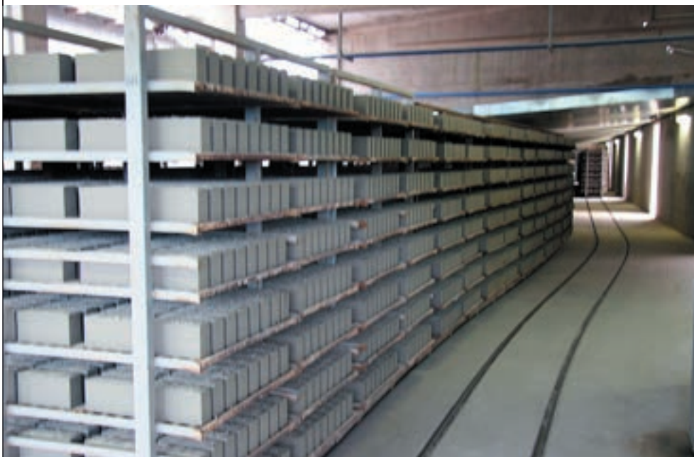
A line of pressed bricks on their way to be dried, fired and machined.
